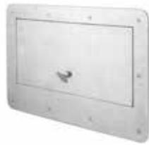
The secure tray hatch is a high secure unit that is installed into doors to provide a secure tray serving solution. Manufactured to allow items up to 14" wide to be passed into a room removing the requirement for the door to be opened for communications or patient serving. Secured with security bolts from the fascia on staff side and no visible screws on patient side.
