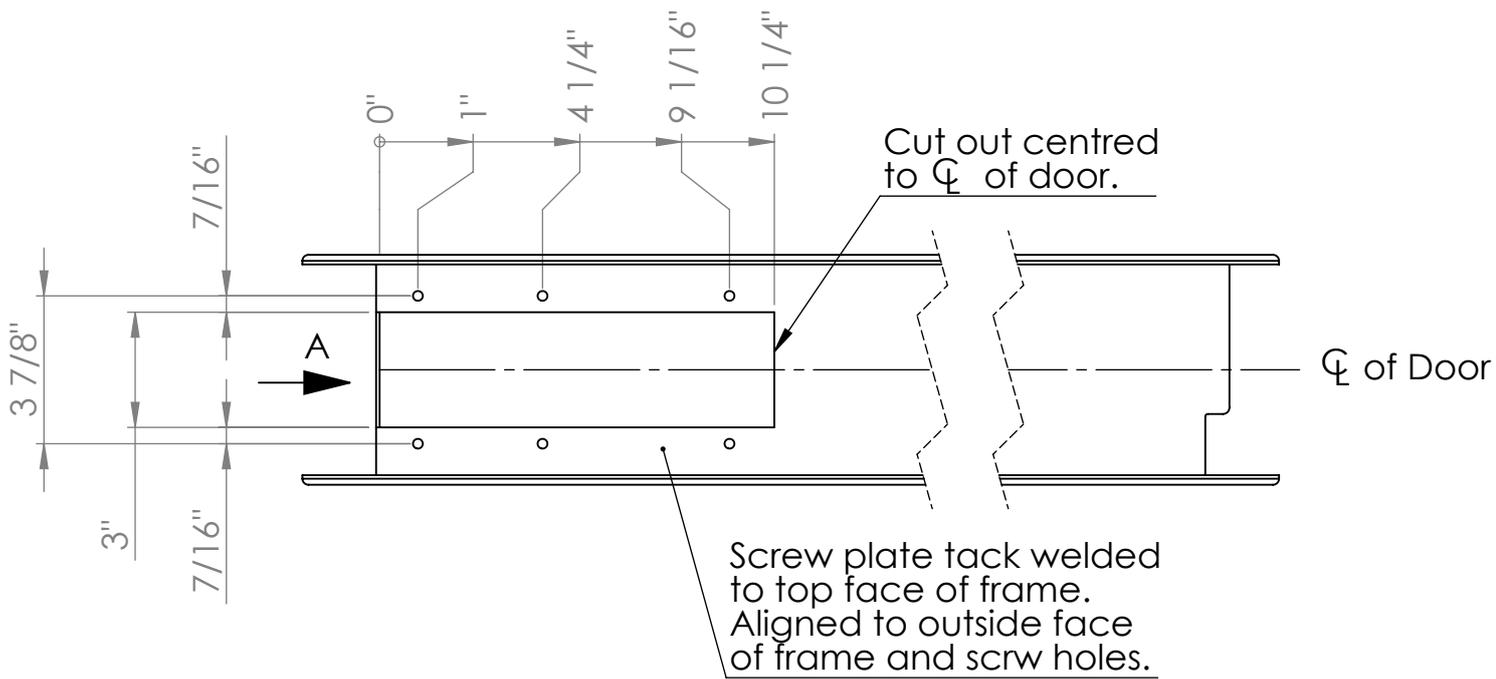
Cut out must go though side profile as well as top profile. Door closer overhangs the frame.
