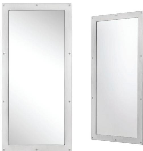
Ligature resistant, shatter proof mirror. Made from an aluminum frame with a polycarbonate mirror center pane. Unit is fixed to the wall with (16) security screws supplied.
