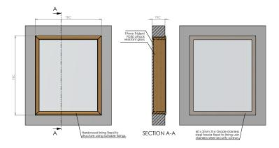
Panorama is a secure glazed screen system. To the patient side there is a stainless steel flush-mounted fascia, the hardwood liner is supplied to suit the wall depth and then finished with a bull-nose detail to the staff side.
