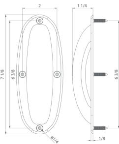
The KG30 Easy Grip pull handle on back plate is made from high-grade stainless steel and is anti-ligature by design. It is designed to be compact and give an excellent grip while remaining safe for secure environments. This handle is supplied with security screws for installation.
