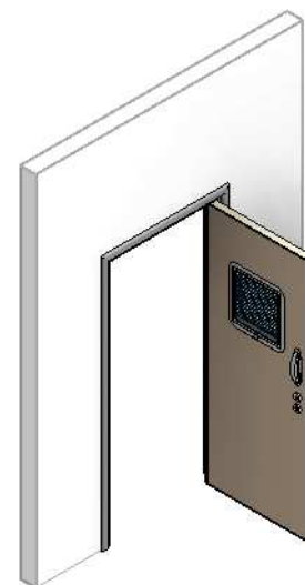
Fig.2 - 3D view of the Kingsway Swing Doorset in the open position. The family provides the ability to view the door in closed or open positions in 3D views without the need for creating additional family types.
